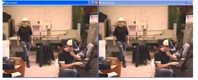
Fig. 3. Sample image frame input on left image, with output regions overlay on right image. This sample illustrates where the intense light induced a specularly, causing the classifier to lose track of the hat.
