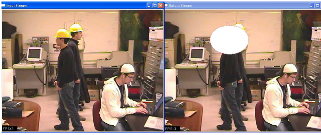
Fig. 4. Sample image frame input on left image, with output regions overlaid on right image. This sample illustrates tracking during a crossing, showing how the Particle Filter grows to accommodate both hats.
