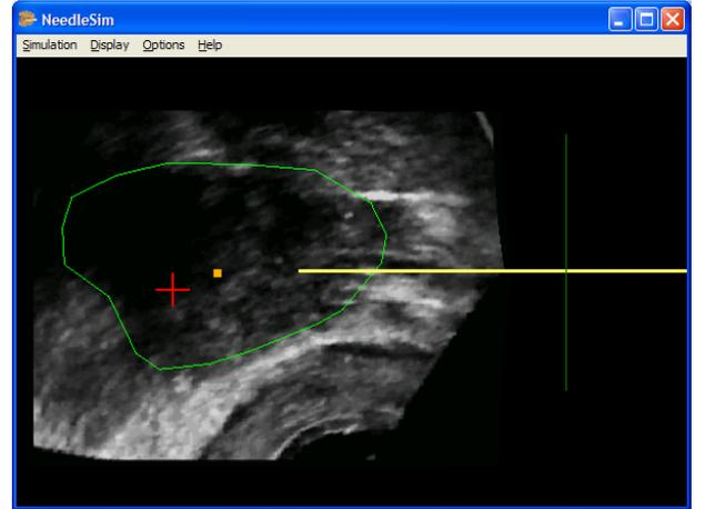
Fig. 4. The simulation user interface, which is based on an ultrasound image, is intended to mimic the experience of a physician performing brachytherapy. The physician interactively guides the needle using a mouse and implants seeds (small squares). Tissue deformations and seed locations are predicted and displayed. The implantation error is the distance between the seed and its target (cross) after needle retraction.
