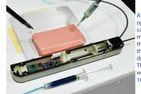
At left: The injector opened to show the carriage for a mounted syringe, the actuation, and the stepper-motor drive board. This device fuctions with 3mL, 5mL, and 10mL syringes.
