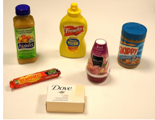
Fig. 5. The first set of objects used for the tests in Section V and Section VI-B. The objects were selected as representative of common household objects and are easily graspable by a parallel-jaw gripper.
